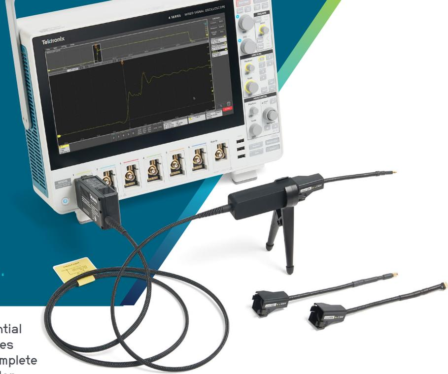
IsoVu probe technology delivers accurate differential measurements up to  $\pm 2500$  V on reference voltages slewing  $\pm 60$  kV at 100 V/ns or faster. Offering complete optical isolation, IsoVu probes reveal signals hidden by common mode noise. They're the industry's first measurement solution to offer a unique combination of high bandwidth, dynamic range, and best-in-class common mode rejection ratio (CMRR) over the probe's full bandwidth.
