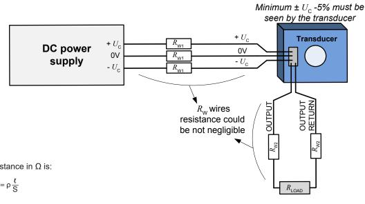
$R_{w}$  wire resistance in  $\Omega$  is:
