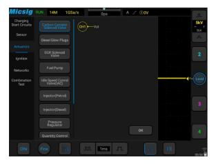
▲ SATO support multiple Actuator tests, including Carbon Canister and EGR solenoid valve, Fuel Pump Injectors, Cooling fan, Pressure Regulator, etc.
