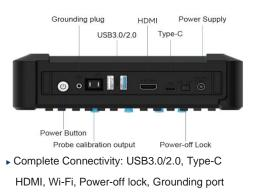
Micsig Universal Probe Interface (UPI), intelligent bi-directional oscilloscope to probe communication, easy to set up attenuation and calibration.
