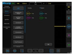
▲ SATO can directly measure the waveform of the sensors, by comparing with standard waveform, it helps user easily find out possible problem.
