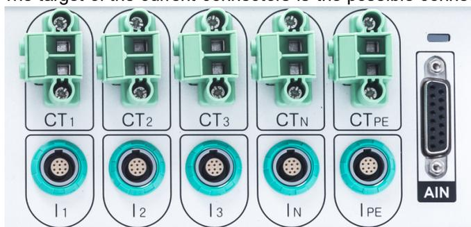
The current can be connected either directly (screw terminals) or with a sensor (Lemo connector).
