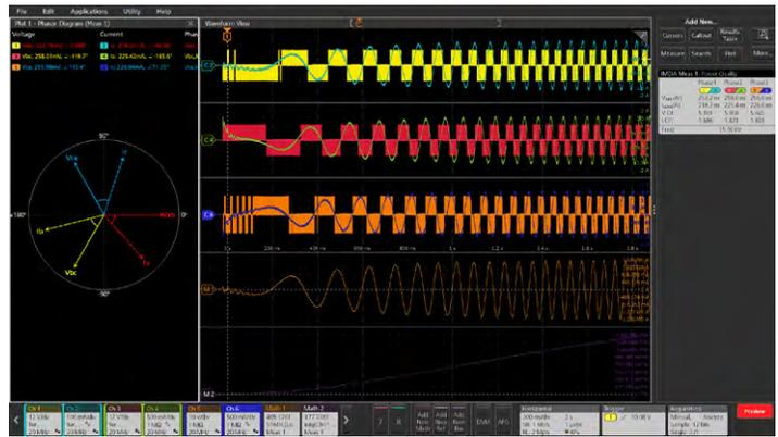
5 and 6 Series MSOs support advanced 3-phase motor drive analysis.
